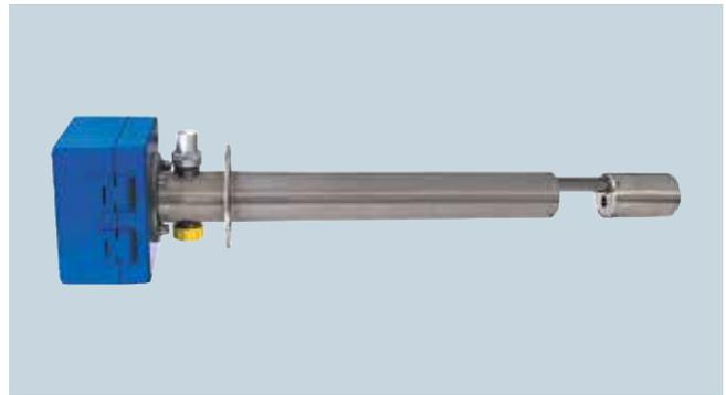
Dust monitor ideally suited for monitoring small to medium dust concentrations. The device uses the forward scattering principle.
