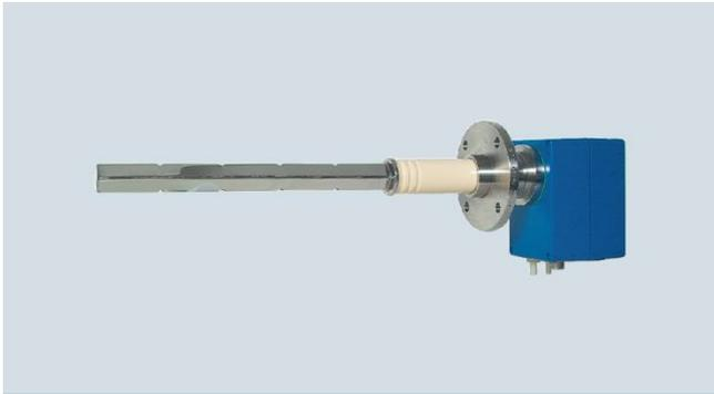
Single rod measurement probe for simultaneous measurement of dust concentration (triboelectric), volume flow, temperature and absolute pressure.
