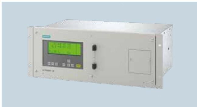
ULTRAMAT 23 is an extremely economical and space saving multi-component gas analyzer also suitable for emission monitoring. It uses NDIR technology for monitoring up to three infrared active components and optionally electrochemical or paramagnetic cell for oxygen measurement.
