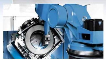
The sealing surface is coated with stellite by a fully automatic welding robot with an integrated measuring system. All CNC programs are developed by our expert in-house programmers. Synchronising the eight axes of the welding system represents a particular challenge.
