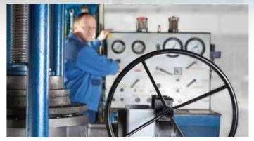
Every ZETRIX® process valve is leak-tested according to DIN EN 12266. The test pressures and times are stored on our computer aided test bench. Special tests can also be performed at the customer's request.
