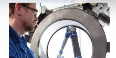
The three-dimensional measuring system allows the process valves to be compared with 3D data, which is subsequently evaluated and saved on a PC. The measurements are carried out directly in the machine to ensure reliable production processes.
