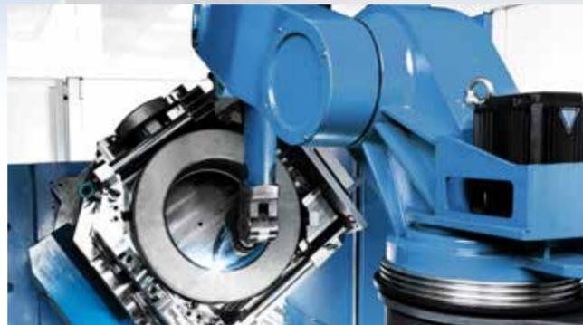
The sealing surface is coated with stellite by a fully automatic welding robot with an integrated measuring system. All CNC programs are developed by our expert in-house programmers. Synchronising the eight axes of the welding system represents a particular challenge.
