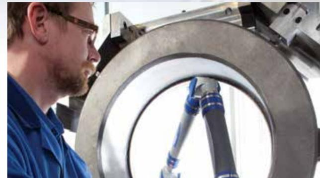
The three-dimensional measuring system allows the process valves to be compared with 3D data, which is subsequently evaluated and saved on a PC. The measurements are carried out directly in the machine to ensure reliable production processes.
