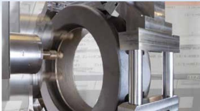
The valve bodies are manufactured on fully automated, CNC controlled machining centres. Our CNC programs are written on the basis of CAD data and transferred to the control online. The workpieces are clamped in specially designed fixtures that guarantee maximum machining stability and short set-up times.
