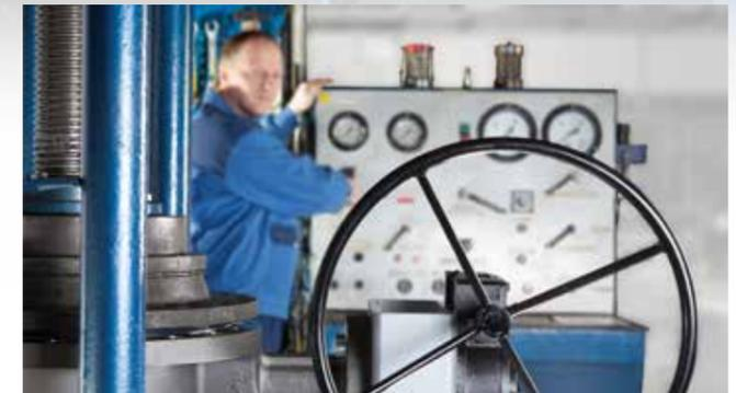
Every ZETRIX® process valve is leak-tested according to DIN EN 12266. The test pressures and times are stored on our computer aided test bench. Special tests can also be performed at the customer's request.
